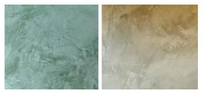
The ultimate look is determined by the consecutive coats. If each coat is applied smoothly, the result will be smooth in colour and structure. If, in the final coat, the irregularities are filled and the whole is polished after setting, this will produce a tadelakt-look. If desired, mixes of several colours can be applied.
